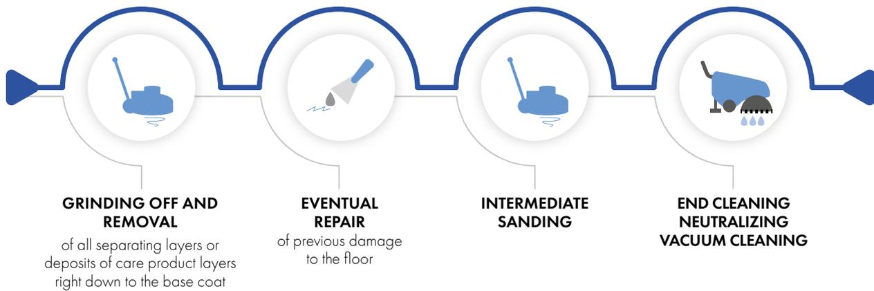
The surfaces of the floors to be sealed **must** be free of any substances which may act as release agents (e.g. waxes, fats, etc.) and in particular must be free from old coatings. Elastic floors must be thoroughly cleaned and wooden floors must be sanded ready for sealing.
